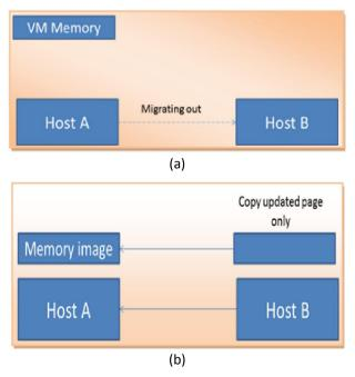
Fig. 2. (a) migrating out from host A to host B. (b) process of memory reusing while migrating back to the same host
