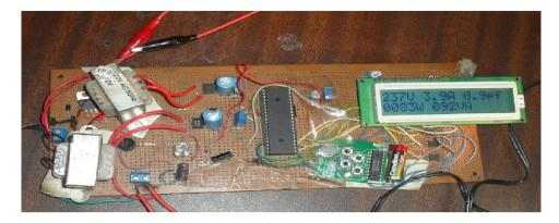
Fig.4: Energy Meter and Transmitter
