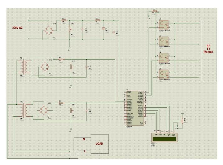
Fig.2: Circuit diagram of an Experimental Work of Energy Meter and Transmitter side
