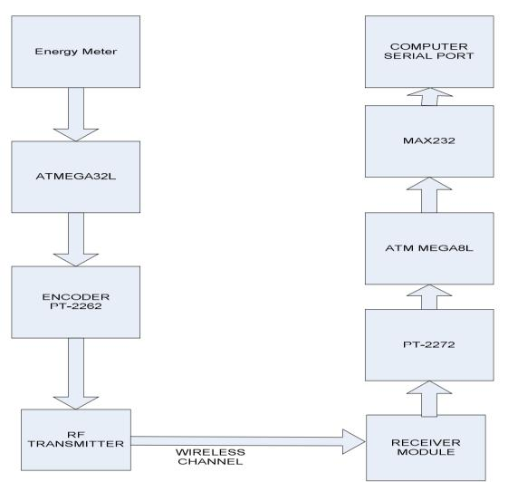
Fig.1 Block Diagram of Experimental Work
