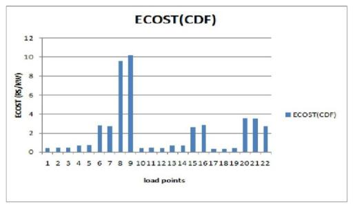
Fig. 4. Calculation of load point ECOST using sector CDF
