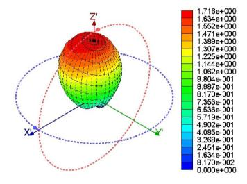
Fig. 5. Far field pattern for 7.49GHz (C-band).
