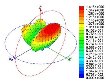
Fig. 7. Far field pattern for 15.70GHz (Ku-band).
