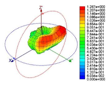
Fig. 8. Far field pattern for 20.10GHz (K-band).
