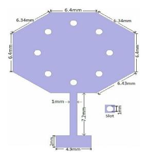
Fig. 1. Proposed compact microstrip patch antenna
