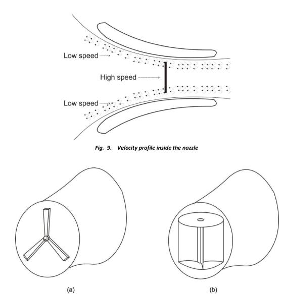
Fig. 10. The condition of the blade area facing the approaching wind in the shroud device(a) The horizontal turbine (less blade area)(b) The vertical turbine (more blade area)
