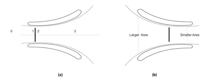
Fig. 2 (a) Model of diffuser shroud wind turbine (b) Nozzle shroud wind turbine
