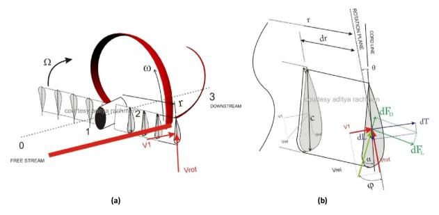
Fig. 3. (a) The model of Blade Element Momentum (b) The detail of the forces on a blade element Illustrated by Rachman, adopted from [6 and 15]
