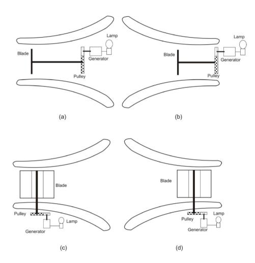
Fig. 4. Models of the wind turbine (a) Horizontal turbine with diffuser (b) Horizontal turbine with nozzle (c) Vertical turbine with diffuser (d) Vertical turbine with nozzle
