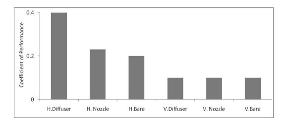
Fig. 6. The Coefficient of performance in the wind models tested
