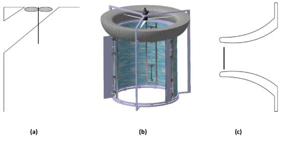
Fig. 1 (a) The shrouded wind turbine in a building section (b) The bucket shape wind turbine (c) The diffuser shroud wind turbine
