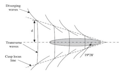
Fig. 1. Ship generated wave model
