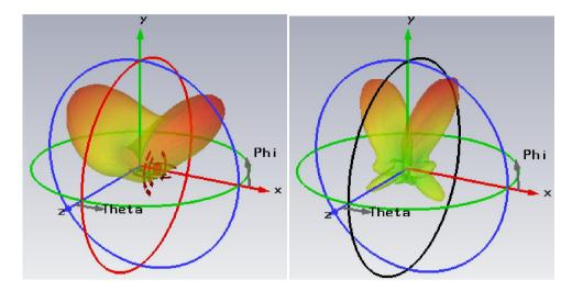
Fig. 4. (a): directivity of antenna for downlink band (b): directivity of antenna for uplink band
