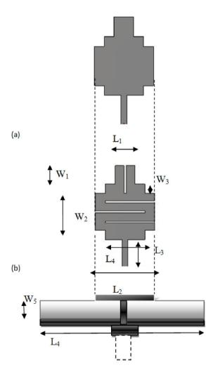
Fig. 1. (a) Basic antenna (b) Modified antenna with slots (proposed)
