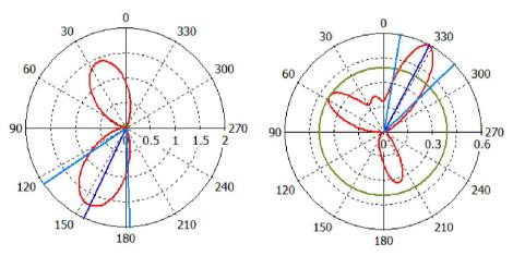
Fig. 5. (a): gain of the proposed antenna for downlink application (b): gain of the proposed antenna for uplink application
