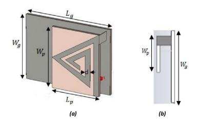
Fig. 2. Proposed triangular Meander – Line Antenna (a) Perspective view, (b) Side view
