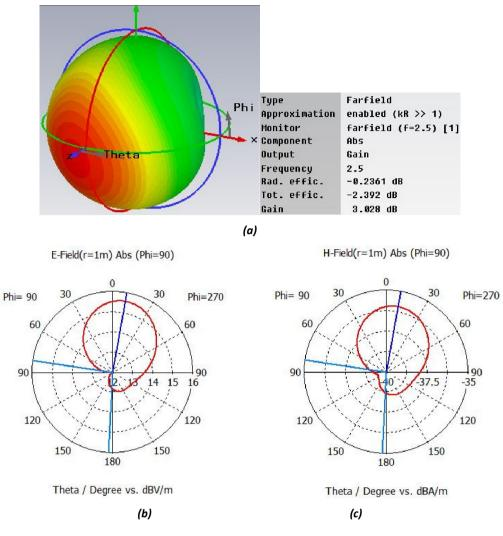
Fig. 4. (a) 3-Dimensional Radiation Pattern, (b) E-field Pattern, (c) H-field Pattern
