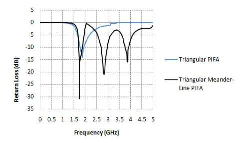
Fig. 3. Comparison between S-Parameter pattern of Triangular PIFA and Triangular Meander-Line PIFA
