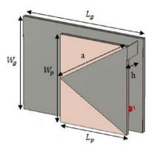
Fig. 1. Triangular PIFA Antenna
