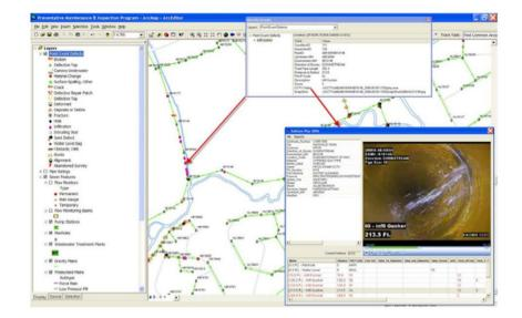
Fig. 5. TV inspection footage is hyperlinked for multimedia viewing within the mapping software
