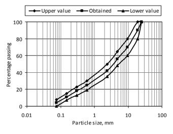
Fig. 1. Gradation of aggregate
