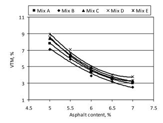
Fig. 3. Voids in total mix of asphalt-concrete with different filler materials
