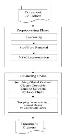
Fig. 2. Block Diagram of the proposed method in web document clustering
