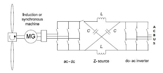
Fig. 6. Z-source based variable speed wind energy systems
