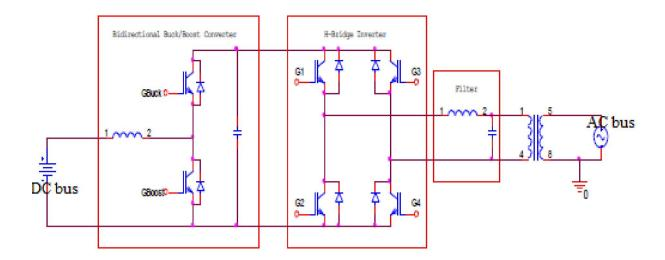
Fig. 8. Circuit diagram of Bi- directional Inverter
