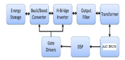
Fig. 7. Bi- directional Inverter block diagram
