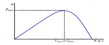
Fig. 3. Typical P-V curve of a PV panel
