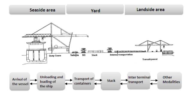
Fig. 1. Processes at a container terminal
