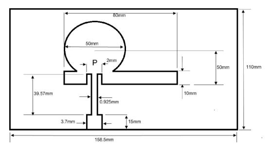
Fig. 1. Geometry of the P-shaped wearable patch antenna
