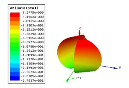
Fig. 3. 3D view of polar plot of the proposed P shaped wearable antenna
