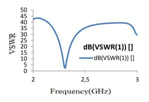
Fig. 5. Simulated result of VSWR at 2.45GHz
