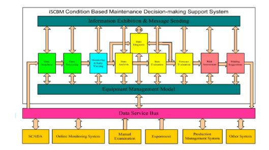
Fig. 3. Diagram of Software Functions of Condition-based Maintenance Decision-making Support System
