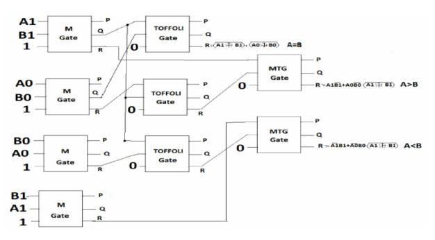
Fig. 4. Architecture for Reversible 2 bit Comparator unit
