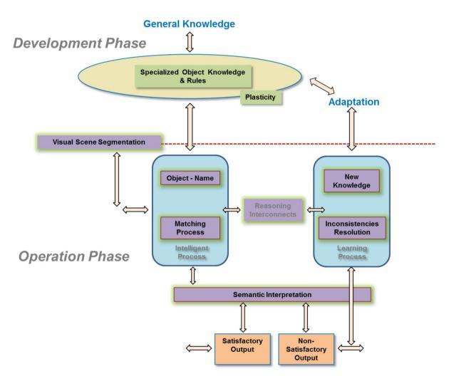
Fig. 11. The Semantic Image Analysis, using a Symbolic Neural Architecture
