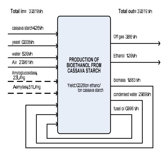
Fig. 1.3 Input-Output diagram for Bioethanol Production from Cassava Starch
