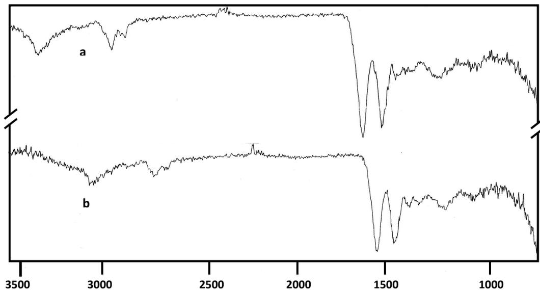
Fig.6 IR spectra of wool/polyamide fabric, (a) untreated, (b) air plasma treated fabric for 10 min., at 10 mA.
