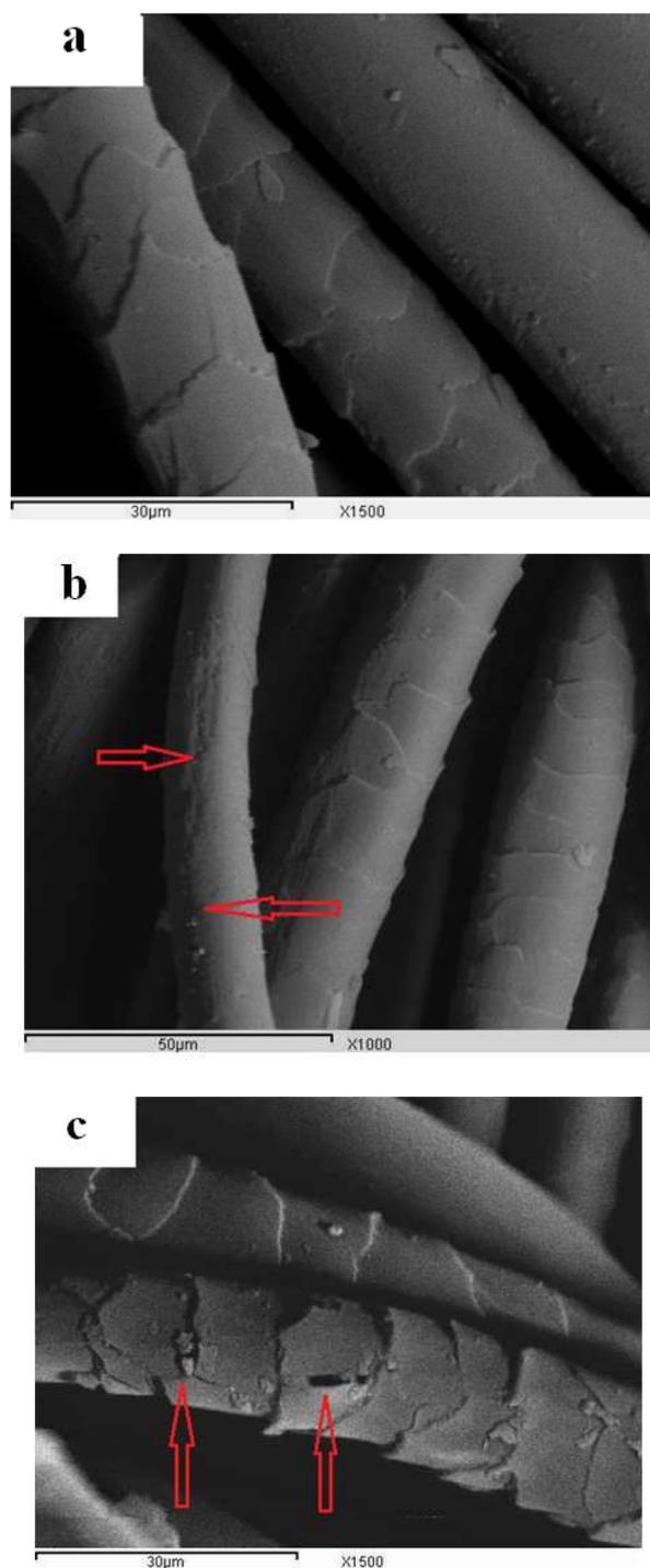
*Fig.5 SEM pictures of (a) untreated, (b, c) air plasma treated wool/polyamide samples at 10 mA for 10 min.*
