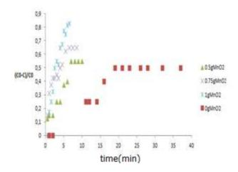
Fig.4 Effect of MnO2 on oxalic acid ozonation [O3]=43mg/l; DO2=21.6l/h; T=25°C;pH=4.3
