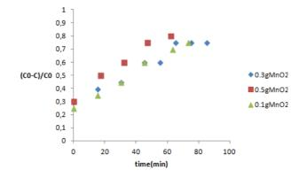
Fig.5 Effect of MnO2 on oxalic acid ozonation [O3]=10mg/l; DO2=21.6l/h; T=25°C;pH=4.3
