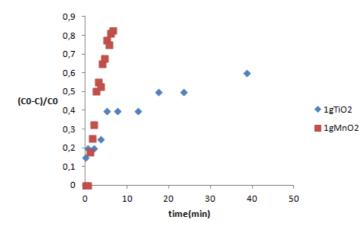
Fig.7 Ozonation of oxalic acid with MnO2 and TiO2 as catalyst, [O3] =43mg/l; DO2=21.6l/h; T=25°C; pH=4.3
