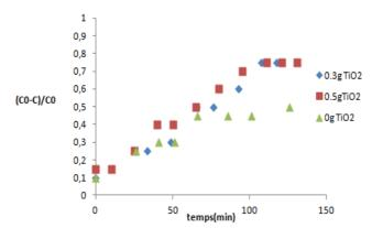
Fig.6 Effect of TiO2 on oxalic acid ozonation [O3]=10mg/l; DO2=21.6l/h; T=25°C;pH=4.3
