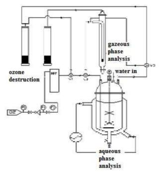
Fig. 1. Installation used for degradation of oxalic acid
