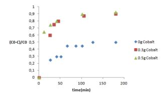
Fig.8 Effect of Co on oxalic acid ozonation [O3]=10mg/l; DO2=21.6l/h; T=25°C;pH=4.3
