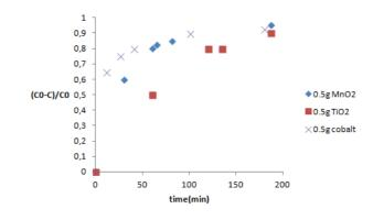
Fig.9 Ozonation of oxalic acid with MnO2 and TiO2 and Co as catalyst, [O3] =10mg/l; DO2=21.6l/h; T=25°C; pH=4.3
