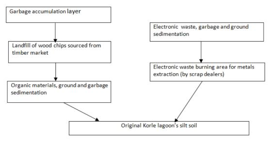
Fig. 6. Solid Waste Accumulation Layers [38]
