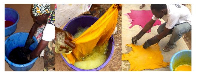
Fig. 3. Dyeing of leather (left), Washing of leather (middle) and Drying of leather (right)
