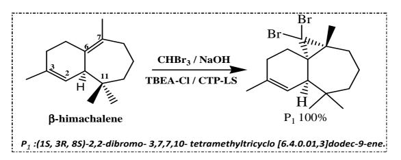
*Fig. 1.* Cyclopropanation Reaction between the β- himachalene and dibromocarbene
