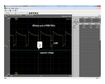
Fig.10 Inductor and capacitor response at 20% dutycyle of PWM of 10kHz
