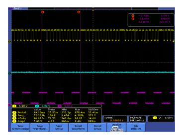
Fig.8 Response of proximity sensor on detection of a tooth of an encoder disc
