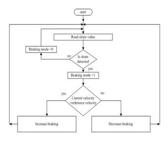
Fig.3. Braking control strategy flowchart
