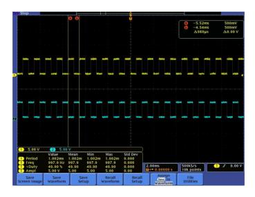
Fig.6. PWM generation of 1kHz and 50% duty cycle
