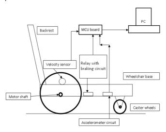
Fig.1. Experimental setup of proposed system
