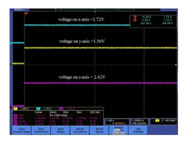
Fig.4. Accelerometer output voltages on three axes in static acceleration mode
