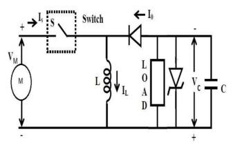
Fig.2. Primary regenerative braking circuit
