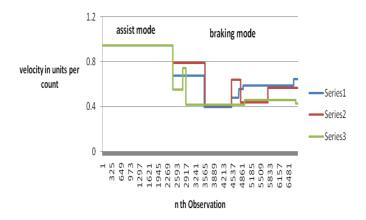
Fig. 12 Velocity pattern of wheelchair for multiple trials on 7 degree declined road
