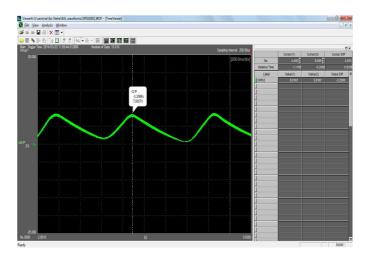
Fig.7. Voltage generated at motor terminals by applying external torque
