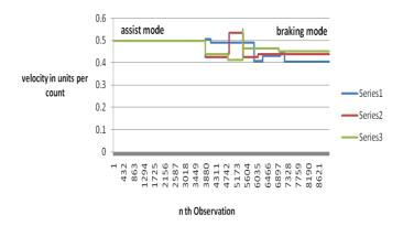
Fig.14 Velocity pattern of wheelchair for multiple trials on 8 degree declined road
