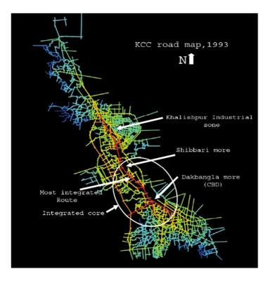
Fig. 6. Axial Analysis of Khulna City Master Plan, 1993
