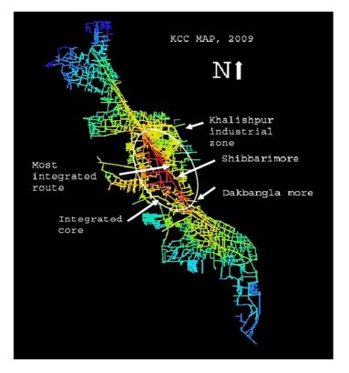
Fig. 7. Axial Analysis of Khulna City Master Plan, 2009
