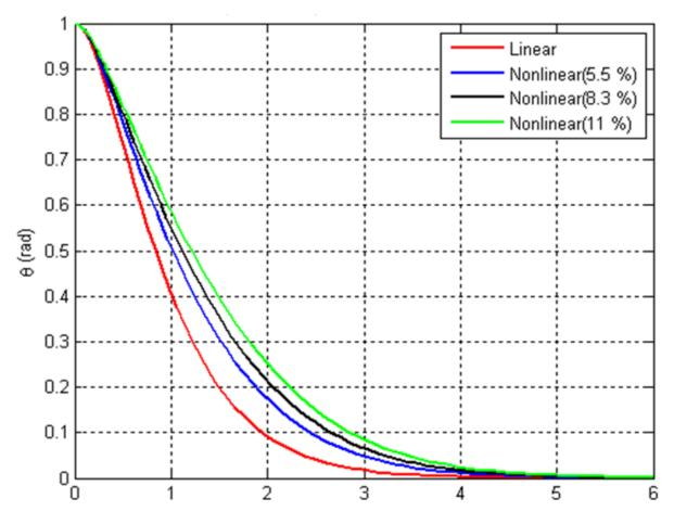
Fig.5 Door response with nonlinear positive deviation.
