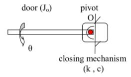
Fig. 1. Automatic door closing mechanism.
