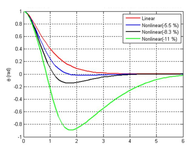
Fig.4 Door response with nonlinear negative deviation.
