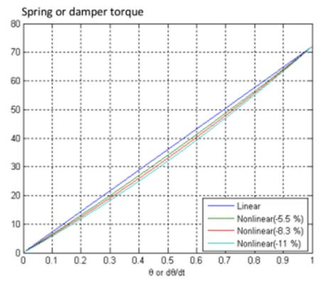
Fig.2 Closing mechanism characteristics (negative deviation)
