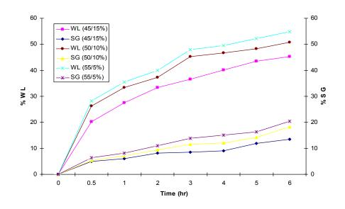
Fig.3.8 Water loss and solid gain of ginger slices with time in different concentration sucrose/salt solution
