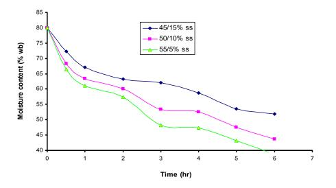
Fig.3.6 Change of moisture content of ginger slices with time in different sucrose/salt solution
