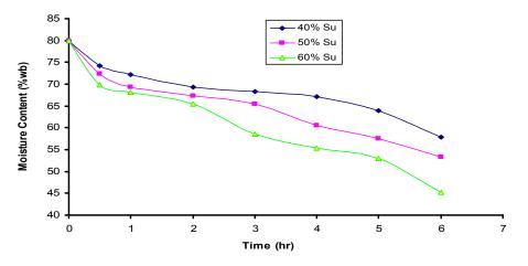
Fig.3.5 Change of moisture content of ginger slices with time in different sucrose solution
