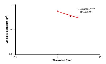
Fig.3.4 Effect of thickness on drying rate constant of ginger slices
