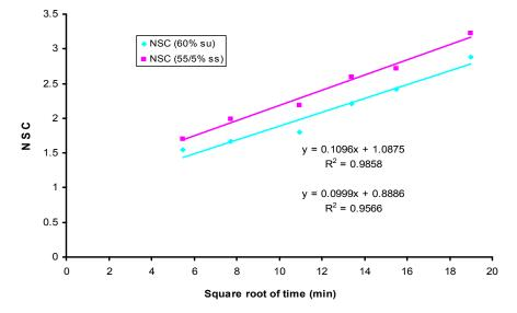
Fig.3.11 Effect of square root of time on normalized solid content for 60% sucrose & 55/5% sucrose/salt solution
