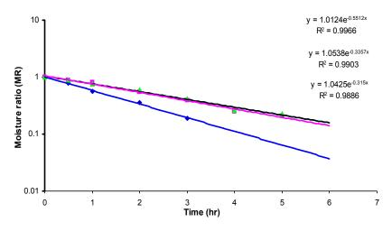
Fig.3.3 Effect of thickness on drying rate of ginger slices
