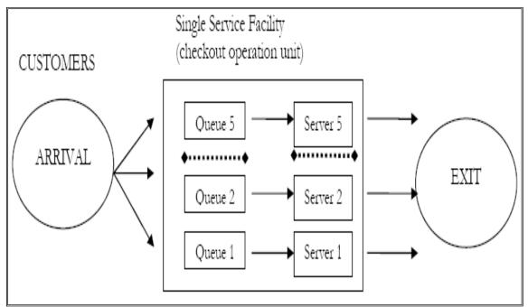
Figure 3: Single Stage Queuing Model With Multiple –Queue And Multiple Parallel Servers
