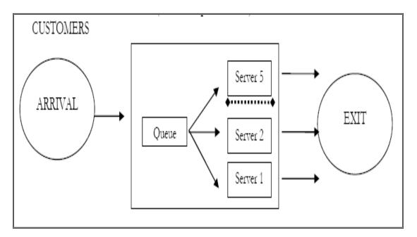
Figure 3: Single Queuing Model With Single –Queue And Multiple Parallel Servers
