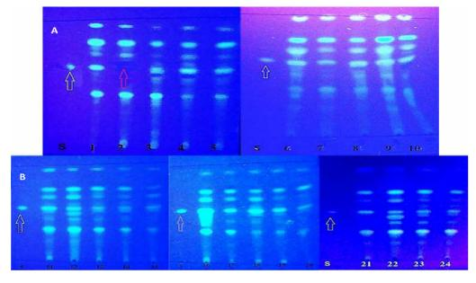
Fig. 1. TLC plate (Silica gel G60 10x5cm) under UV light (336 nm) illustrated AOH samples and standard spot by using development solution (toluene-ethyl acetate-90% formic acid (5: 4: 1 v /v).
