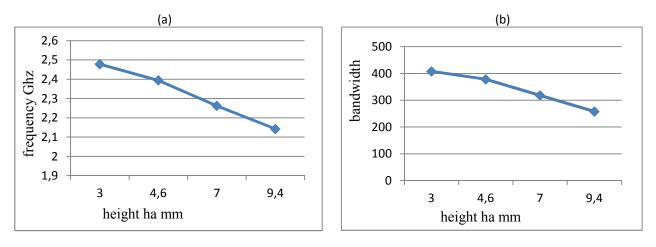
Fig. 6. Changes of the height ha according resonance frequency and bandwidth
