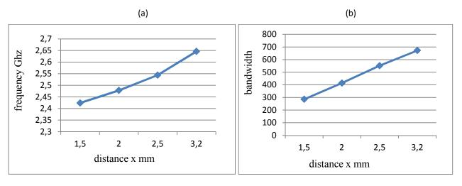
Fig. 7. Changes of the distance x according resonance frequency and bandwidth
