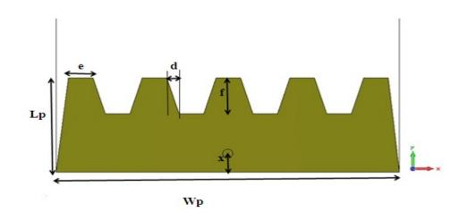
Fig. 2. the geometry of the top radiating plate
