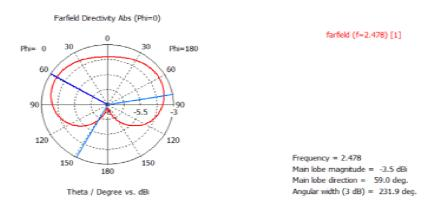
Fig. 8. Simulated radiation patterns in dB ( $\varphi = 0$ , x-z plane) at fr=2.478 GHz
