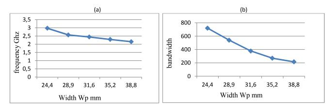
Fig. 4. Changes of width of the radiating plate according resonance frequency and bandwidth
