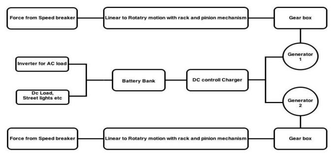
Fig. 5. Block diagram of PGS
