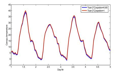
Figure 6. The effect of cover longwave emission coefficient on canopy temperature
