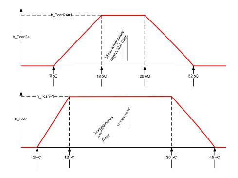
Figure 1.Temperature growth inhibition factor computation method
