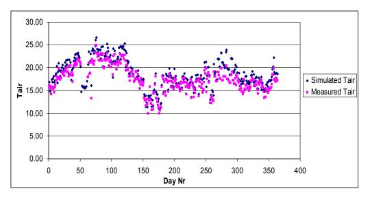
Figure 2. Comparison of simulated and measured mean daily greenhouse temperature
