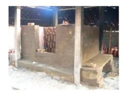
Figure 13. Open vessel furnace with firewoods
