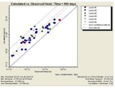
Fig 2. Head calibration for unlined canal
