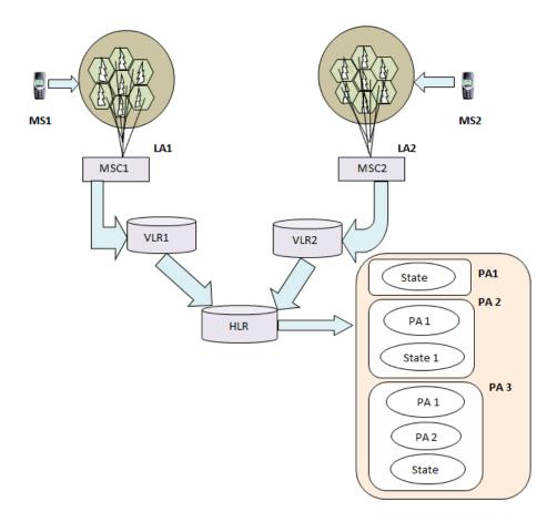
Figure 1: MSIP-GSM Architecture
