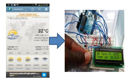
Fig. 2. Temperature calibration between android application and Robot temperature sensor
