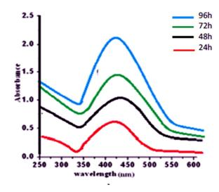
Figure (1): UV-Visible spectroscopy of silver nanoparticles with peak at 440 nm
