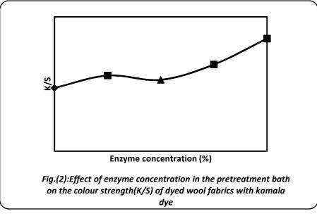
**Pretreatment:** L.R: 1:50, at pH=7, and at 70° C for 60 min. **Dyeing:** L.R 1:100, 6% natural dye, 2 g/L dispersing agent and at 80°C for one hour.
