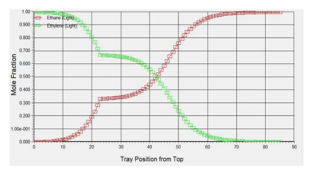
Figure 7: Mole fraction vs tray position from top
