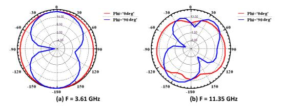
Fig. 9. Simulated radiation patterns of the proposed antenna, (a) f = 3.61 GHz and (b) f = 11.35 GHz
