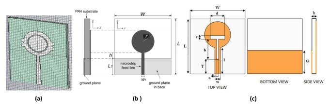
Fig. 10. Geometry of the reference antennas and the proposed antenna, (a) [11], (b) [12] and (c) proposed antenna
