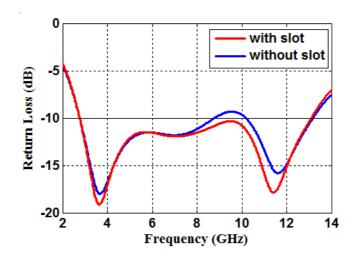
Fig. 2. Simulated return losses of the proposed antenna with and without T-shaped slot
