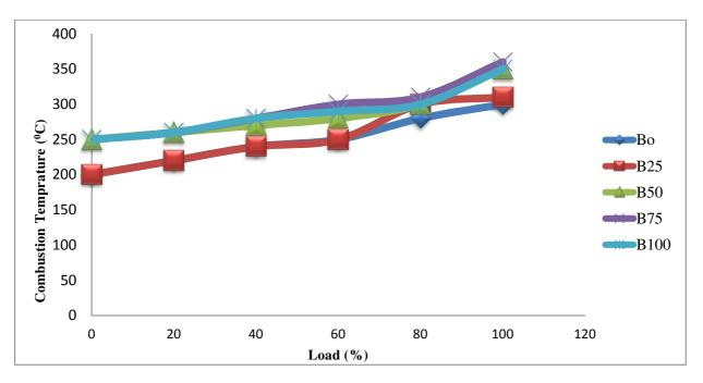
Figure 2. Effects of Methyl Ester and its Blends on Combustion Temperature
