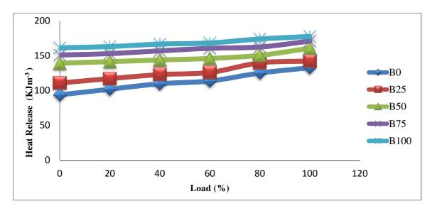
Figure 5. Effects of Methyl Ester and its Blends on Heat Release Rate
