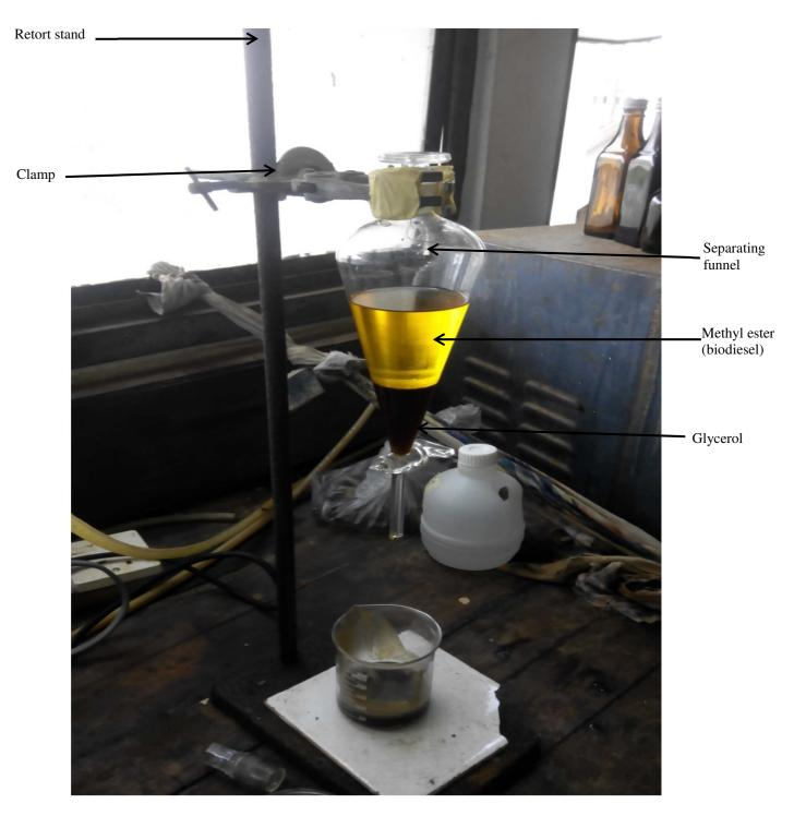
Figure 1. Methyl Ester Separation Using Separating Funnel during Experiment
