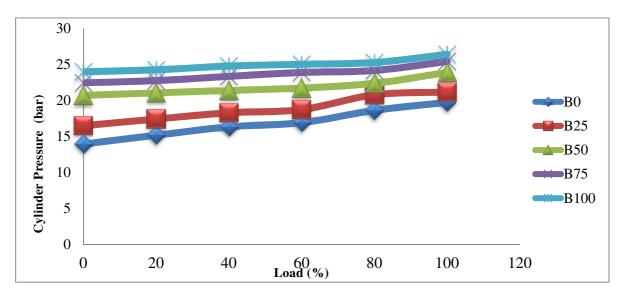
Figure 4. Effects of Methyl Ester and its Blends on Cylinder Pressure
