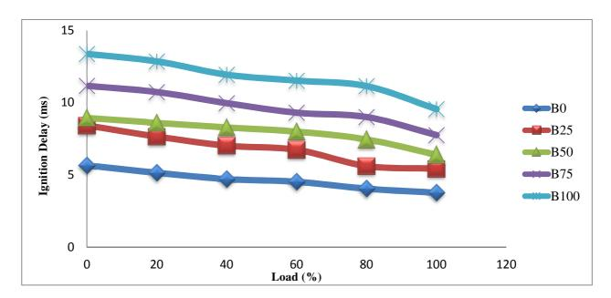
Figure 3. Effects of Methyl Ester and its Blends on Ignition Delay
