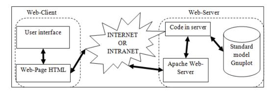
Fig. 3. Data Flow in a Network-Based Application
