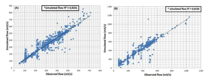
Fig. 7. Simulated versus observed flow, 5 years for calibration (A) and 3 years for validation (B)
