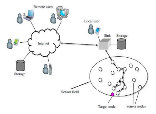
Fig. 1. A Typical Wireless Sensor Network
