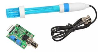
Fig. 4. pH sensor with probe
