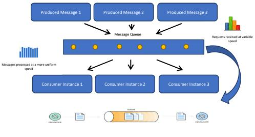
Fig. 5. Message queue with load leveling
