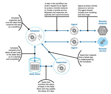
Fig. 8. Logic components of Scheduler Agent Supervisor Pattern
