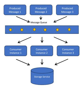
Fig. 7. Asynchronous queue with messages from different producers
