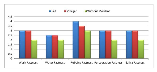
Fig. 1. Comparison of the fastness properties with different mordant
