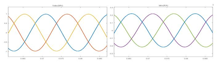
Fig. 9. Voltage and current of the fault-free line
