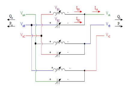
Fig. 5. three-phase model of the RPI30P15 connecting two regions of a network [1]
