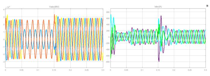
Visualization of voltages and current in the presence of an RPI
