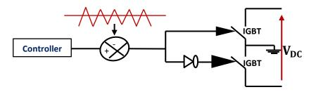
Fig. 7. Principle of the PMW Sinus-Triangle command [15]
