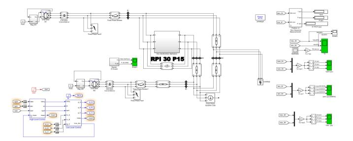
Fig. 15. Faulty network in the presence of the RPI controller
