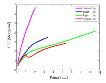
Fig. 4. TEL electronic energy loss as a function of the penetration of the Ar, Kr, Xe and U ions into the silicon
