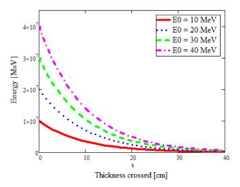
Fig. 11. Profile of the energy deposited as a function of the thickness crossed for X0 = 9.569 cm
