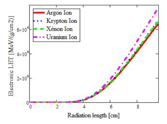
Fig. 10. Electronic LET of Ar, Kr, Xe and U ions in silicon as a function of radiation length
