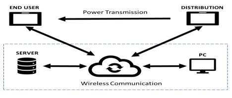
Fig. 5. IoT unit configuration for energy supply and monitoring
