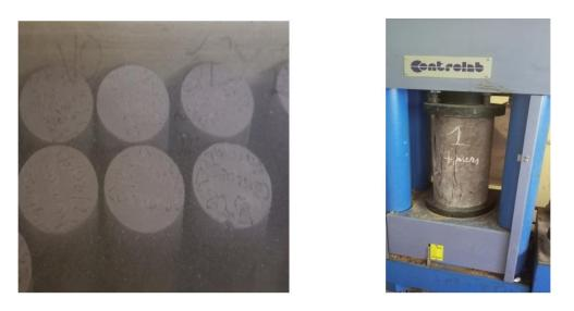
Fig. 2. Preservation and crushing of specimens.
